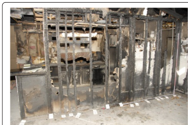
Fig. 1 Wood stud wall with varying DOFD char damage
