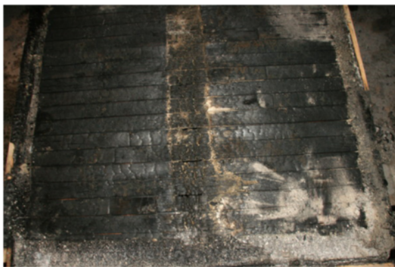
Fig. 9 Resultant floor burn pattern from carpet pad seam without use of ignitable liquids (Wood et al. 2012)
