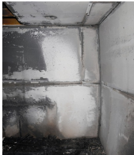
Fig. 11 Photograph of a Plume-Generated Fire Pattern (fire origin was located at the base of this damage-test conducted at EKU by author)
