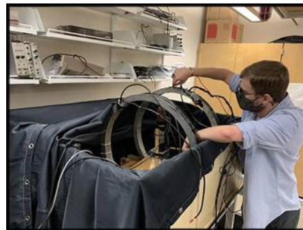
Mr. Jonathan Mills testing the effect magnetic fields have on light collection from a Sodium Iodide (NaI) detector.
